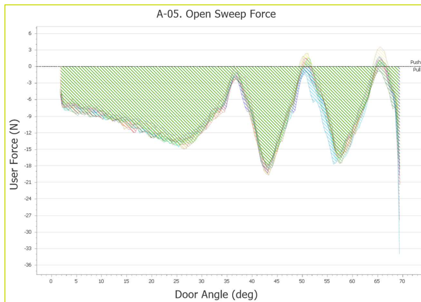
Figure 13: Open Sweep Force: User force for varying door angles
