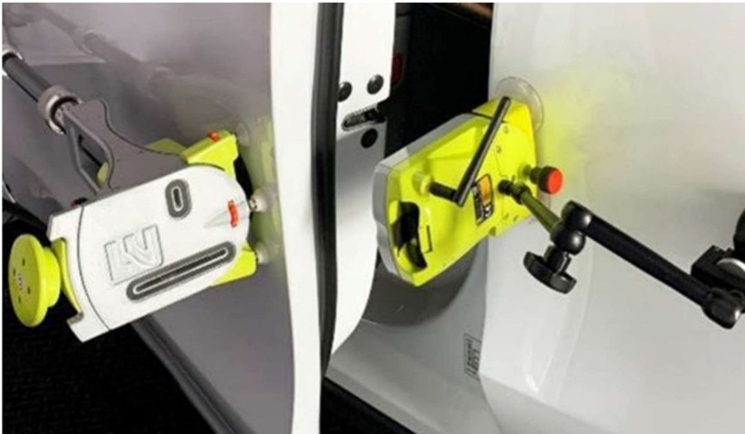
Figure 1: EZSlam installed on automobile door.
